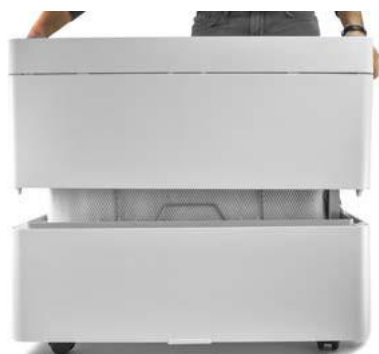
Fig. 7.4.2.1: Removing the upper part of the housing
