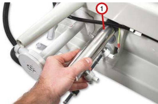
Fig. 8.1.2.5: Remove UV disinfection housing
