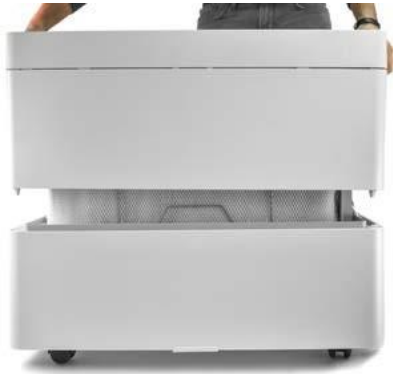
Fig. 8.1.1.1: Removing the upper part of the housing
