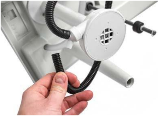
Fig. 7.4.1.5: Pulling off the pump hoses
