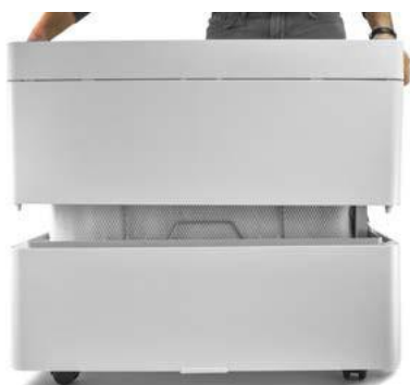
Fig. 6.3.1.1: Removing the upper part of the housing
