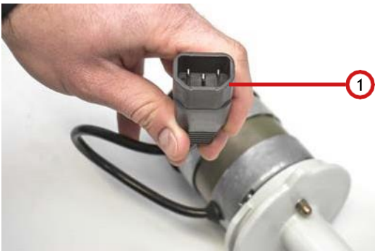
Fig. 7.4.1.7: Loosening the plug connection
