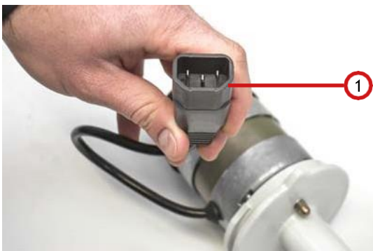
Fig. 7.4.1.7: Loosening the plug connection
