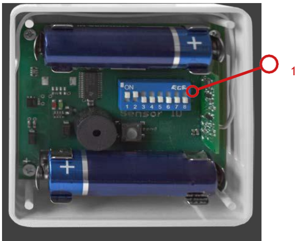
Fig. 5.6.4: Coding the radio humidity transmitter
