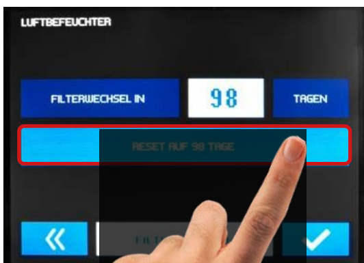
Fig. 6.3.2.7: Reset filter change indicator
