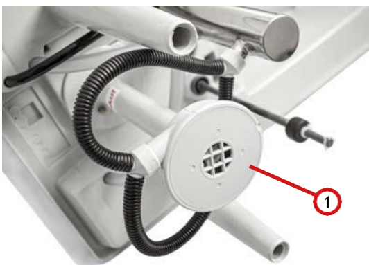
Fig. 6.3.4.6: Cleaning the pump body
