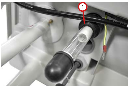
Fig. 8.1.2.6: UV lamp in quartz glass tube.
