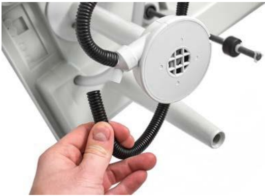
Fig. 7.4.1.5: Pulling off the pump hoses
