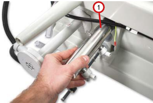
Fig. 8.1.2.5: Remove UV disinfection housing
