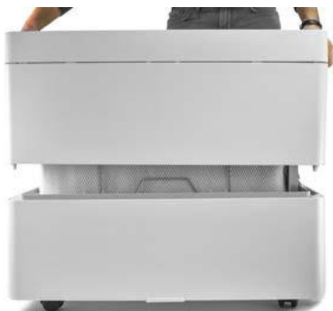
Fig. 7.4.2.1: Removing the upper part of the housing
