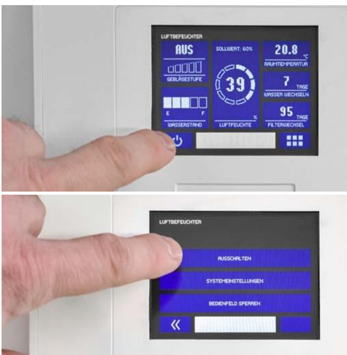
Fig. 5.2.2: Switching off the unit
